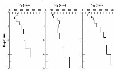
Figure 4. Inverted  $V_{s}% \left( f_{s}^{2}\right) =0$  for (a) Mardyke GAA pitch, (b) Fitzgeralds park and (c) Mardyke bridge
