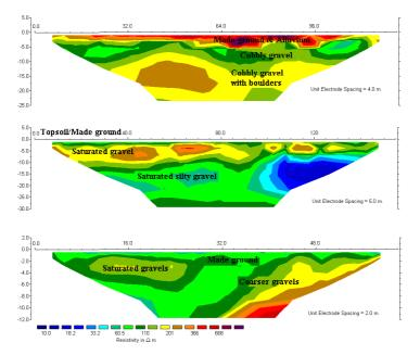
Figure 3. Modelled Resistivity Sections from (a) Mardyke GAA Pitch (b) Fitzgerald's Park and (c) Mardyke Bridge
