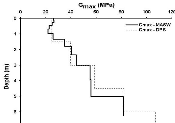
Figure 3:  $G_{max}$  profile for the DPS model comparing the Surfseis (MASW) produced profile with the actual  $G_{max}$  profile created in the DPS
