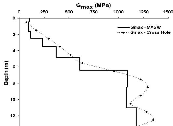
Figure 2.  $G_{\max}$  from MASW compared with corresponding cross-hole survey for St. James Hospital
