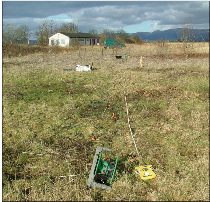
Figure 4. MASW testing at Bothkennar
