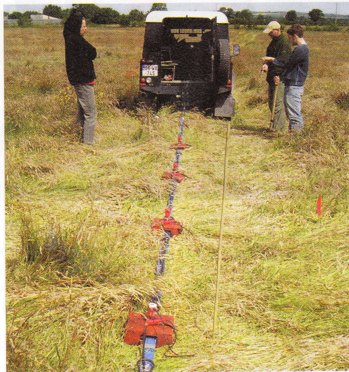
Figure 1: A MASW survey was carried out for the Dublin Metro North project with a 2D V_s profile generated by towing a "streamer" of geophones along the route to collect data every 6m
