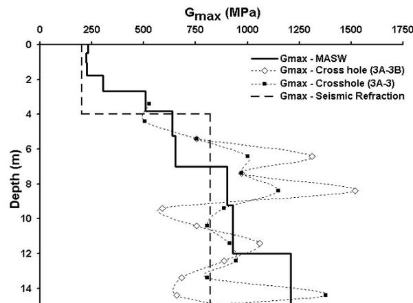
Figure 1.  $G_{max}$  from MASW compared with corresponding cross-hole and seismic refraction surveys for Dublin Port Tunnel
