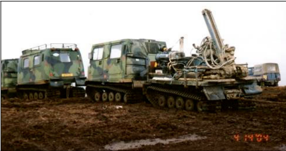
Figure 3. Articulated, tracked vehicle used by the geophysical crew and drillers.
