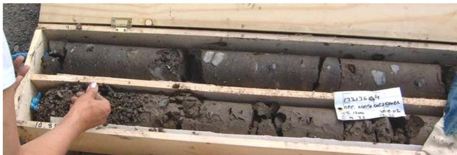
Figure 1: Geobore-S core of Dublin boulder clay showing distinct sand or silt lens within the largely clay matrix (Skipper et al., 2005)
