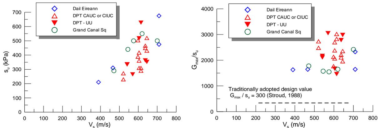
Figure 4: The variation of  $V_s$  with (a)  $s_u$  and (b) the design parameter  $G_{\max}/s_u$
